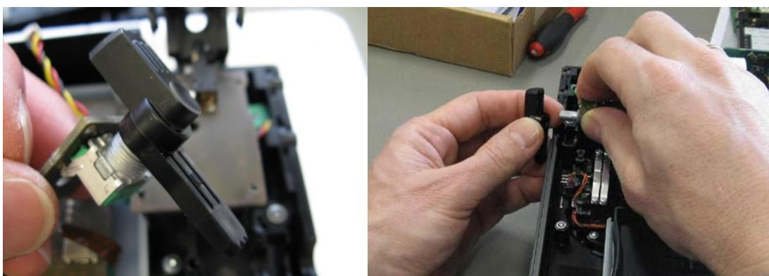
5. Re-fit the side-mounted rotary slider board and fit the retaining screw. Close the case.
